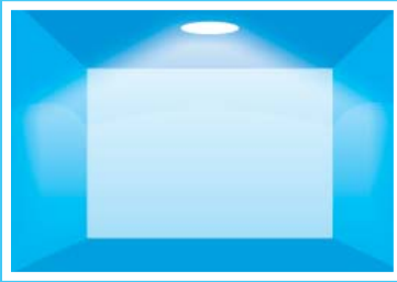
The simplified light distribution shown below the light tunnel installed in the middle of the room without windows.
